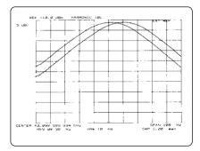
Spectrum analyzer photo of 8341A/8349B/ 83555A signals at 44 GHz with resolution of 10 Hz.
