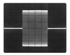
8340A/8349B/83554A pulse performance at 35 GHz. Pulse width = 5 ms.
