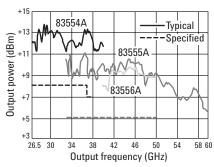
Typical maximum leveled output power available from the 83550-series millimeter-wave source modules.
