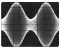
8341A/8349B/83554A AM performance at 30 GHz. AM rate is 17 kHz and depth is 70%.
