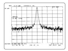
Spectrum analyzer photo of 8340A/8349B/83556A signal at 50 GHz.
